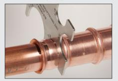
Confirm the finished crimp band diameter by using the RLS crimp gauge. When properly crimped, the RLS crimp gauge allows the marked slot to fit snug on the crimp band. If it doesn't fit, it is undercrimped and will need to be re-crimped. 2. Look for the "RLS"
